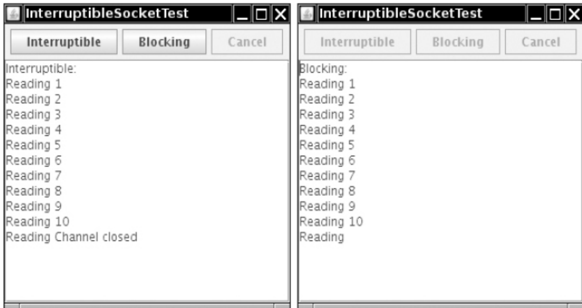
Figure 4.6 Interrupting a socket
